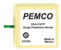
The **PEMCO FAS-31XTP** is a single pair telephone protector that implements an advanced three-stage hybrid design. This unit addresses over-voltage transients with gas discharge tubes (GDT) and silicon breakover devices. Additionally, sneak and fault currents are mitigated with PTC technology, which consists of solid state resettable fuses. FAS-31XTP is specifically designed for more rugged applications such as traffic cabinets.
